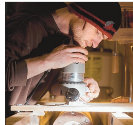
Sean Kelly turns the center column for his next spiral staircase on his custom-built lathe.
